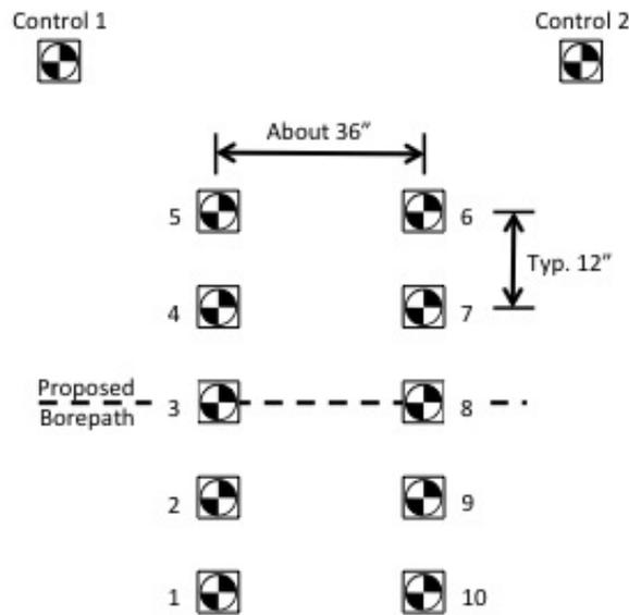
**Figure 1.** Typical Arrangement of Targets on Each Site
