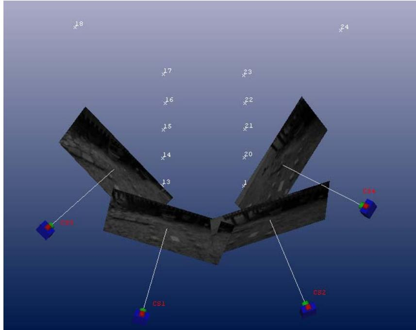
**Figure 3.** Three Dimensional Point Cloud with Camera Stations (Site C-4)
